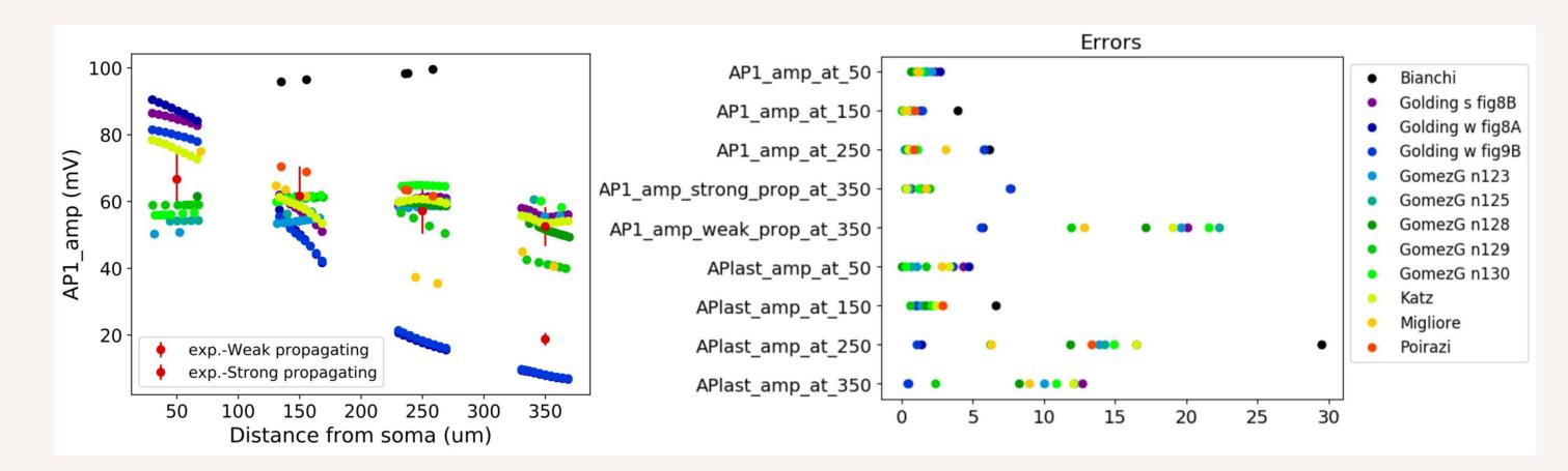
The amplitudes of the first back-propagating action potentials (in an around 15 Hz train) as a function of recording location distance from the soma (left), and Feature error scores achieved by the different models on the Back-Propagating AP Test (right)
